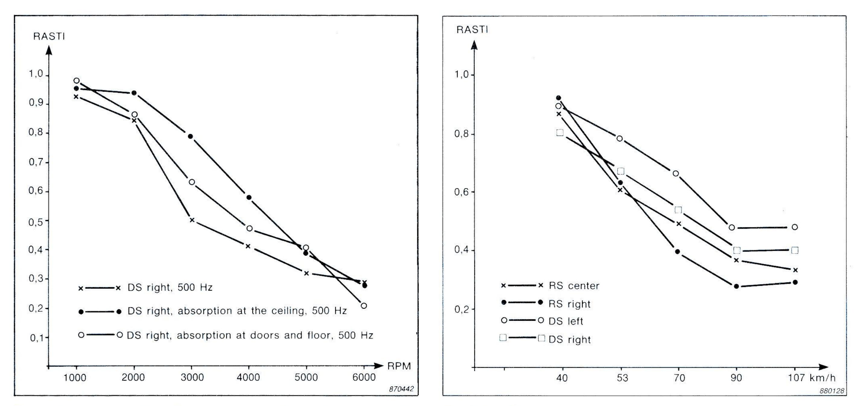
Fig. 4. Results with different kinds of absorption in the cabin for DS right and only for 500 Hz
