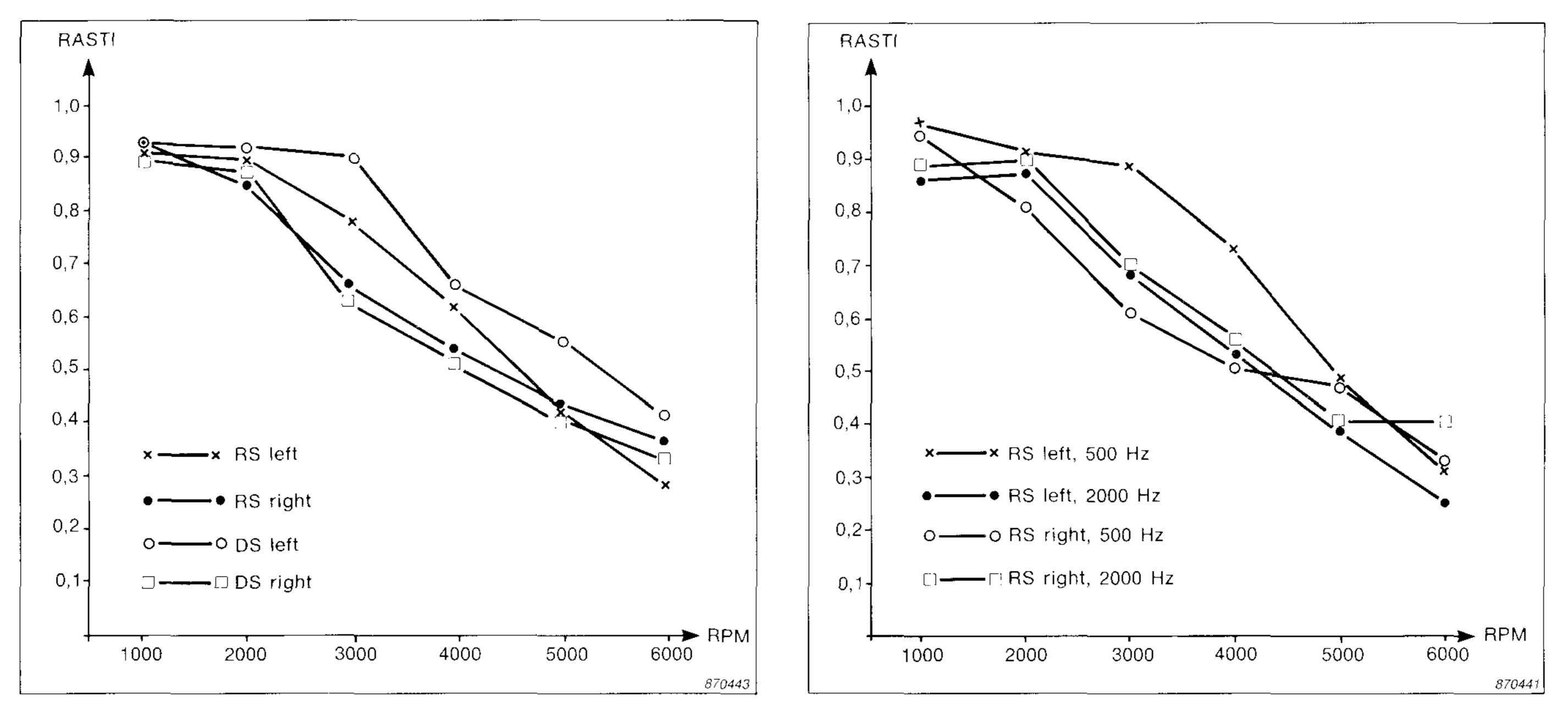
Fig. 2. RASTI results from measurements in a stationary car
